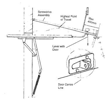
Open the door and using the door centreline to vertically align the screwdrive assembly, prop the unit up such that the drive end cover is level with the door. Ensure that the door's highest point of travel clears the screwdrive assembly.
