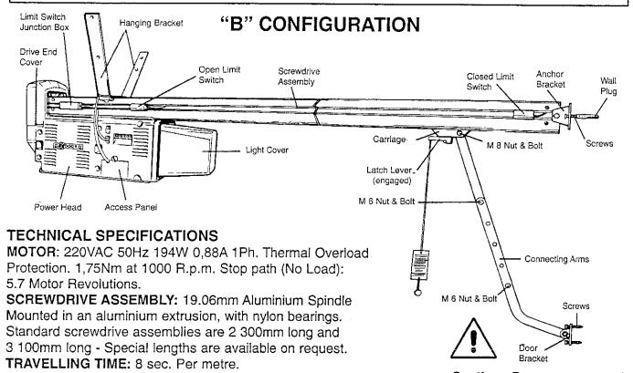
Caution: Damage may result if the connecting arm is forced backwards while only one end is attached to the carriage.
