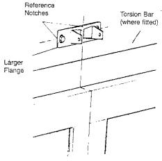
With the door closed, extend and mark the centre line of the door on the wall above the door. Mark the cross line 50mm above the highest point of the top edge of the door in it's travel.
