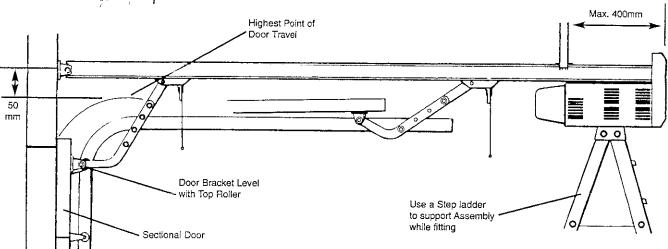
Ensure that the carriage is fitted with the large hole away from the powerhead. Secure the screwdrive assembly to the anchor bracket with the M6 x 75mm bolt provided while supporting the motor end.
