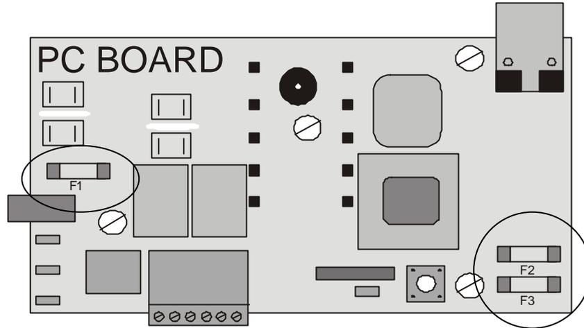
**HOW TO CHECK: (ALL FUSES ARE 2 AMPERE FAST BLOW)**
